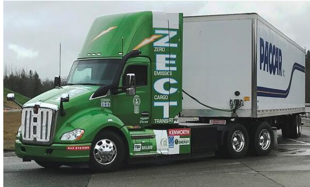
Kenworth T680 Day Cab Drayage Truck powered by Ballard FCveloCity(R)-HD module
